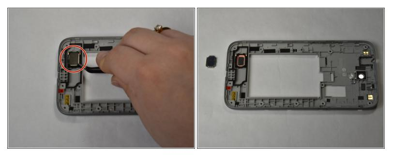
Use the curved tweezers to grab onto one of the corners of the speaker and pull upwards and lift out.
