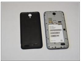
Use the iFixit opening tool to open up the device by wedging the tool under the back case and popping it open.
