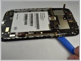
Use the iFixit opening tool to dig under the sticker where the volume and the power buttons are located on both sides.
