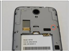
Use a Phillips #00 screwdriver to unscrew all 12 of the 3 mm Phillips screws located along the edges of the device's back panel, as well as the blue 3mm Phillips screw labeled "ZTE" located towards the top right.
