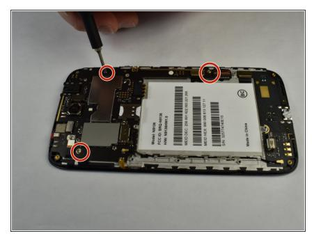
Remove the three 3 mm Phillips #00 screws on the edges of the motherboard.
