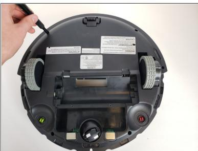
Using a Phillips #00 screwdriver, take out the six screws around the perimeter of the bottom case.
