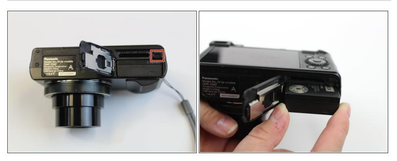
• Push up the black tab on the right-hand-side to spring release the battery.
