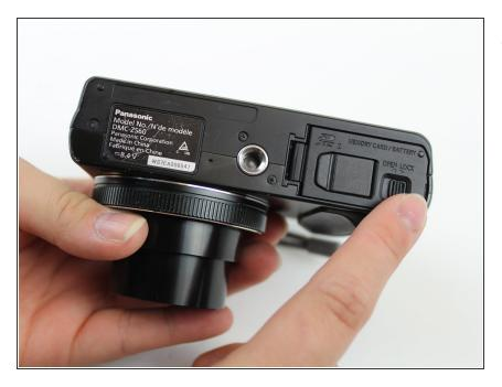
Use your finger to slide the black latch from the locked position to the open position on the memory card/battery door. This will open the door of the camera.
