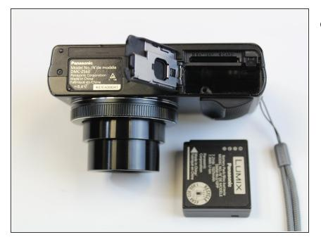
• Remove the battery by sliding it out from the camera.
