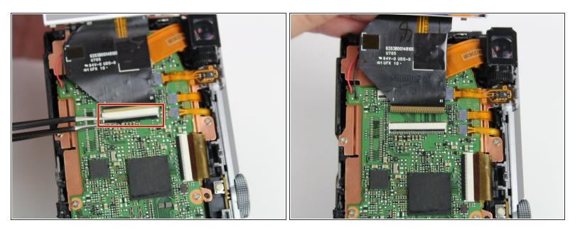
Use tweezers to pry up the black retaining flat and gently pull to free the LCD screen from the device.
