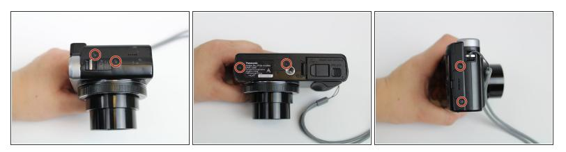
Using the Phillips #000 Screwdriver, unscrew six 3mm screws. There are two screws located on three sides excluding the top.
