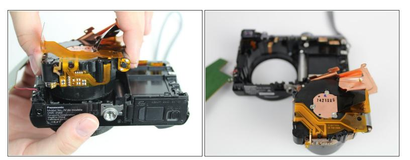
• Lift the camera lens from the camera.
