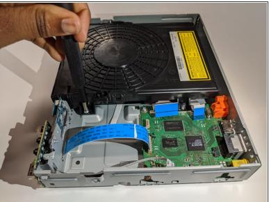
Use a Phillips #2 screwdriver to remove the two 9mm screws that are holding the disk drive in place.
