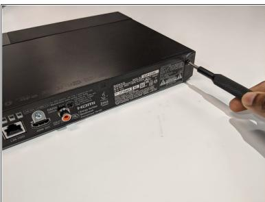
Use the Phillips #2 screwdriver to remove the two 9mm screws located on the back of the device.
