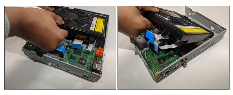
Carefully lift and slide the disk drive out of the casing.
