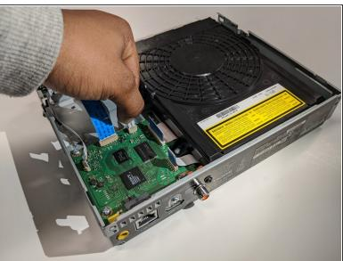
Remove the three ribbon cables by gently pulling the cables out of each connector.
