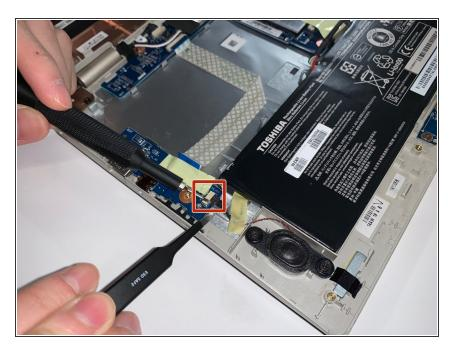
Disconnect the cable that connects the receiver to the laptop using the pointed end of a spudger.
