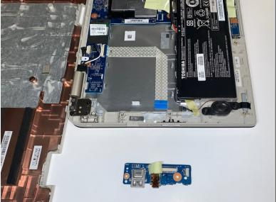
Peel back the material covering this wire.
