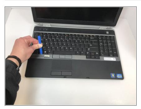
Use the spludger to lift the grey casing off the Dell Latitude E6530 keyboard.
