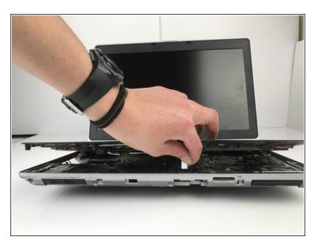
• Lift off the final casing and remove the motherboard.
