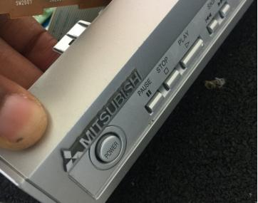
Adjust and push the new button into place.
