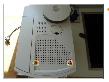
Remove the two Torx T10 screws on the top.
