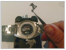
Once the back of the watch is removed, use tweezers to carefully remove the first two plates which are connected.
