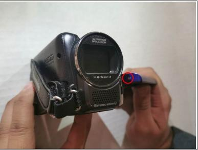
Use a Phillips #00 screwdriver to remove two screws from behind the corners of the display screen.
