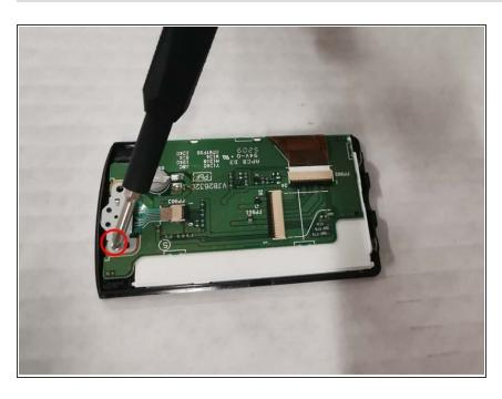
Use a Phillips #00 screwdriver to remove one screw on the green panel.
