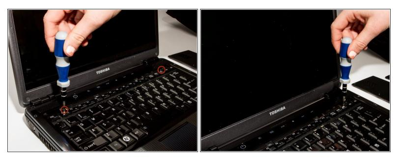
• Using #1 Phillips Screwdriver, remove both of the 5 mm screws that are located beneath the insert.
