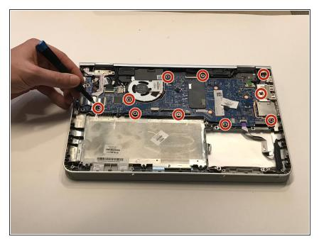
Remove the ten 1.2mm Phillips #1 screws that hold the motherboard into the frame of the laptop.
