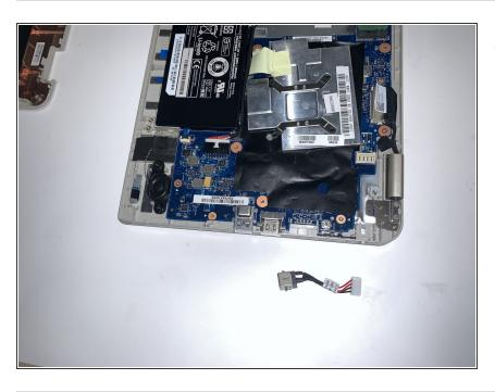
Once the port has been disconnected, carefully lift the whole charging port off the panel.
