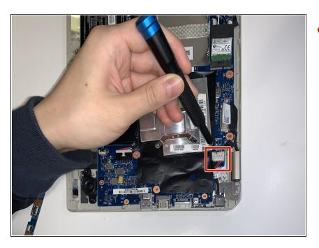
Detach the white connector from the laptop using the pointed end of a spudger.
