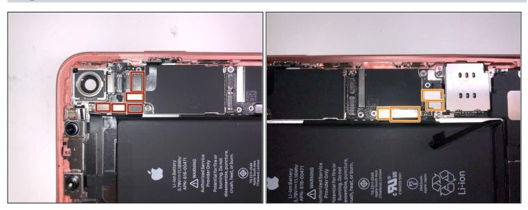
Use an opening tool or a fingernail to remove 9 connectors from the logic board.
