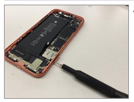
• Use a sim eject tool or a paperclip to remove the SIM tray.
