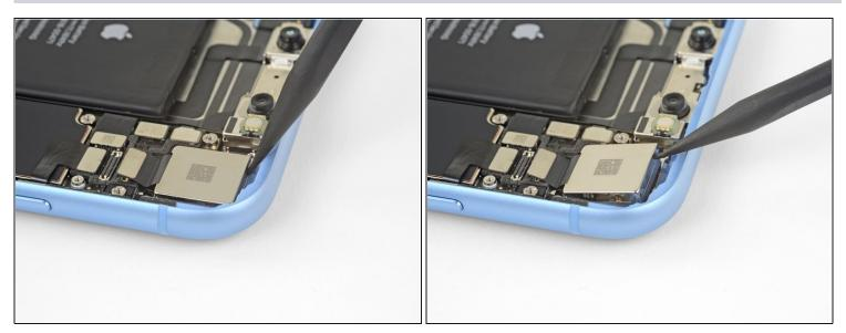
• With a spudger, gently pry up on the camera to remove the camera.
