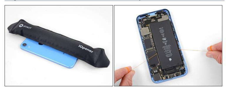
• If any of the adhesive strips broke off and the battery remains stuck to the rear case, <u>prepare an iOpener</u> or use a hair dryer to heat the rear case directly behind the battery. This will help soften the adhesive.
