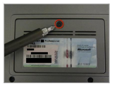
Locate and unscrew the captive screw indicated in the picture on the left to detach the panel.
