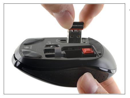
If the Nano Receiver is still in the mouse and not in your computer, remove it by pushing on the bright orange button. It should pop right out!
