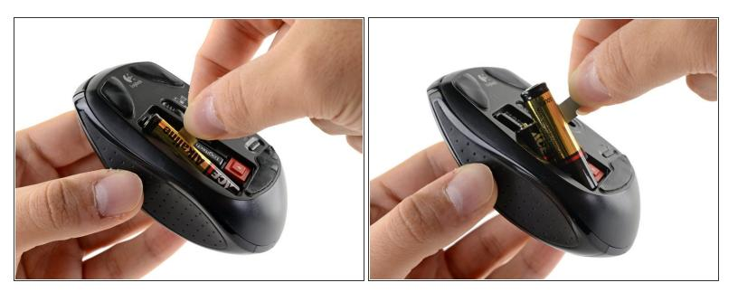
• Pull the battery release tab away from the mouse so the two AA batteries come out.
