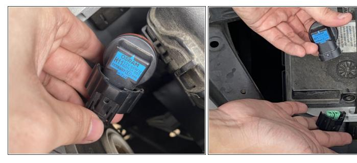
Hold onto the bulb with one hand while holding down the clip at the bottom of the plug to remove the bulb.
