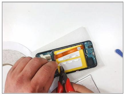
• Use Double side Adhesive tape to install the battery to the new frame
