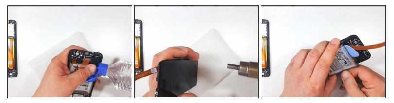
• To remove the Battery use a few drops of alcohol and warm the device.
