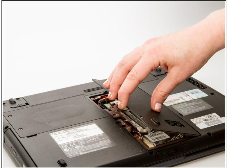
**!** After removing the screw in step 3, carefully close the laptop and put it face down. Locate the center panel.
