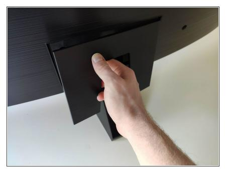
• Remove the cover at the base at the back
