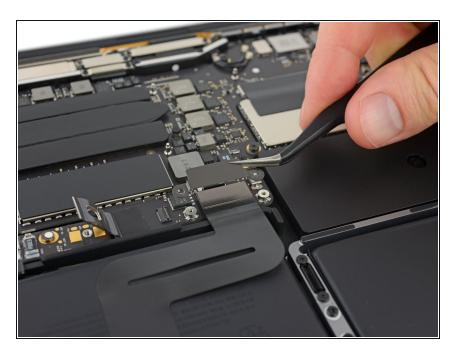
Remove the trackpad cable connector bracket.
