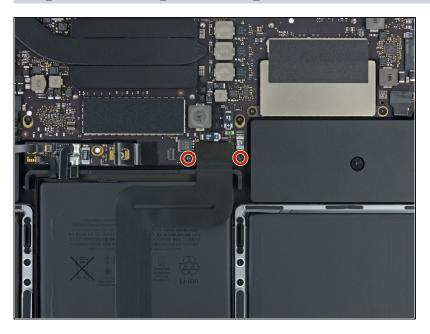
Use a T5 Torx driver to remove the two 2.1 mm screws securing the trackpad cable connector bracket.
