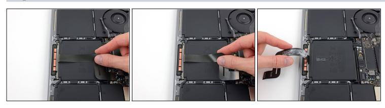
• Carefully peel the trackpad ribbon cable up off the battery, and push it out of the way.
