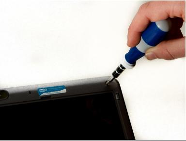
Use a #1 Phillips screwdriver to remove the 3mm screws located on both sides of the top of the laptop as well as the lower corners.
