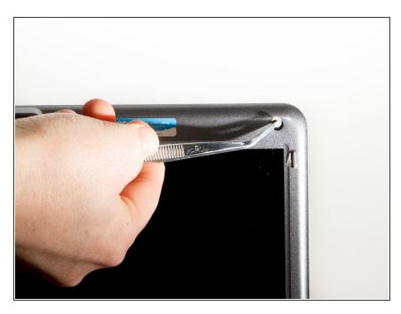
Use tweezers to remove the small rubber covers over the screws on the top and bottom of the laptop case.
