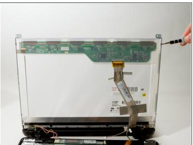
Locate and remove the four 2mm #1 Phillips screws around the sidewalls of the display.
