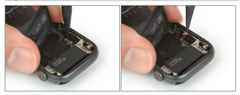
• Use the pointed end of a spudger to pry up and disconnect the battery flex cable.
