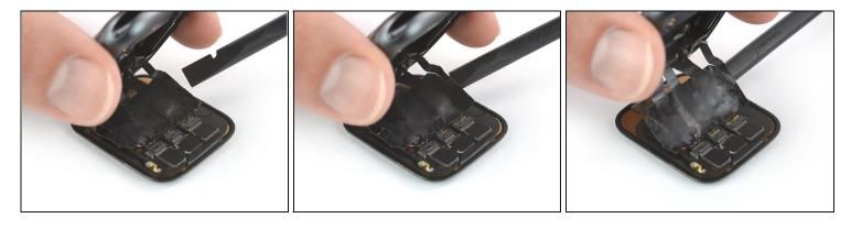
• Lift the body of the watch up and carefully slide a spudger underneath the display flex cable to loosen remaining adhesive.
