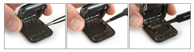
• Use a pair of blunt nose tweezers to peel up the sides of the black foil which adheres the cable to the rear side of the screen.
