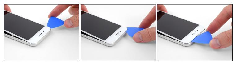
• Slide an opening pick underneath the display around the top left corner and along the top edge of the phone to loosen the last of the adhesive.
