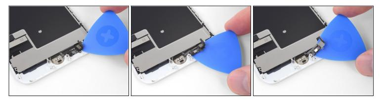
• Use an opening pick to gently separate the adhesive holding the home/Touch ID sensor cable to the back side of the display panel.
