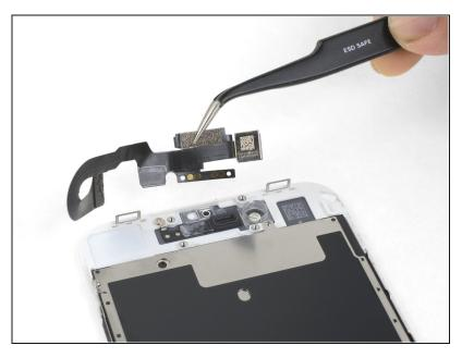
Remove the front camera and sensor cable.
