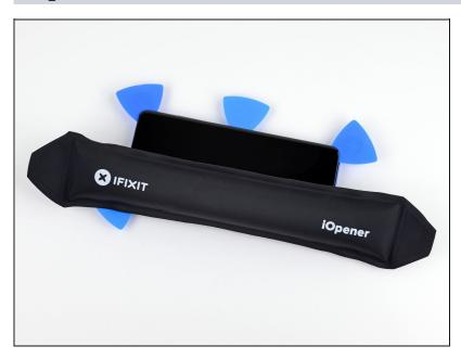
Apply a heated iOpener to the left edge of the display for two minutes.
