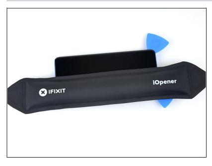
Apply a heated iOpener to the right edge of the display for two minutes.
