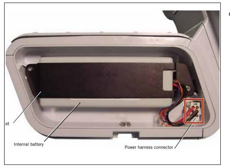
Disconnect the internal battery from the power harness connector.
