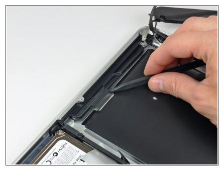
• Use the tip of a spudger to pry the right speaker up off the adhesive securing it to the upper case.
