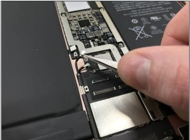
• Use tweezers to disconnect the antenna connectors.
