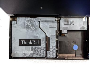
Lift the battery using it's cloth pull tab and lift it out of the ThinkPad. Set it aside.
