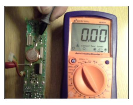
Using a voltmeter, measure the voltage of the battery. The voltage should be around 3.0 volts.
