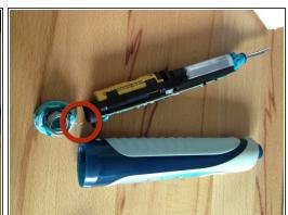
Push the bottom of the toothbrush against the knob on the back of the charger. Turn counter clock wise and the bottom should pop off. Put the toothbrush top down on a hard surface and push the inner part out.
