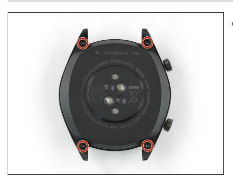
Remove the four Torx T3 screws (3.65 mm length).
