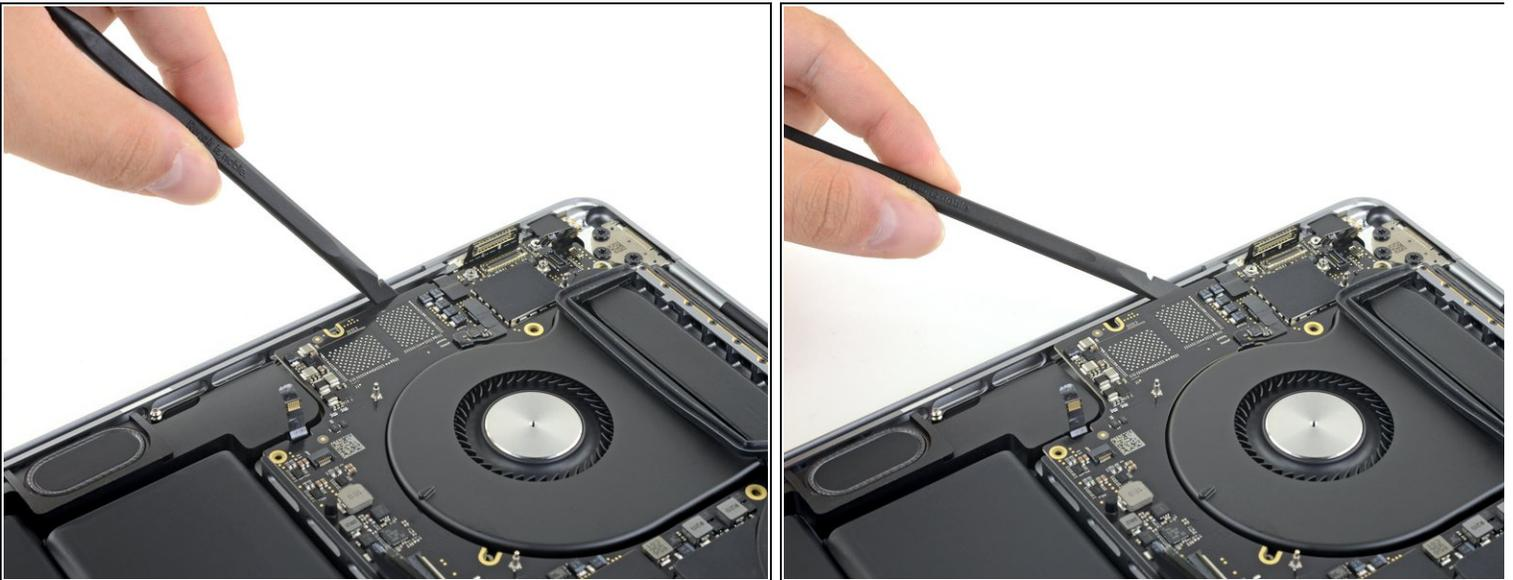
**i** The logic board assembly is a tight fit, but you can make it easier to remove by inserting a spudger under the left edge and levering it up **slightly**.
