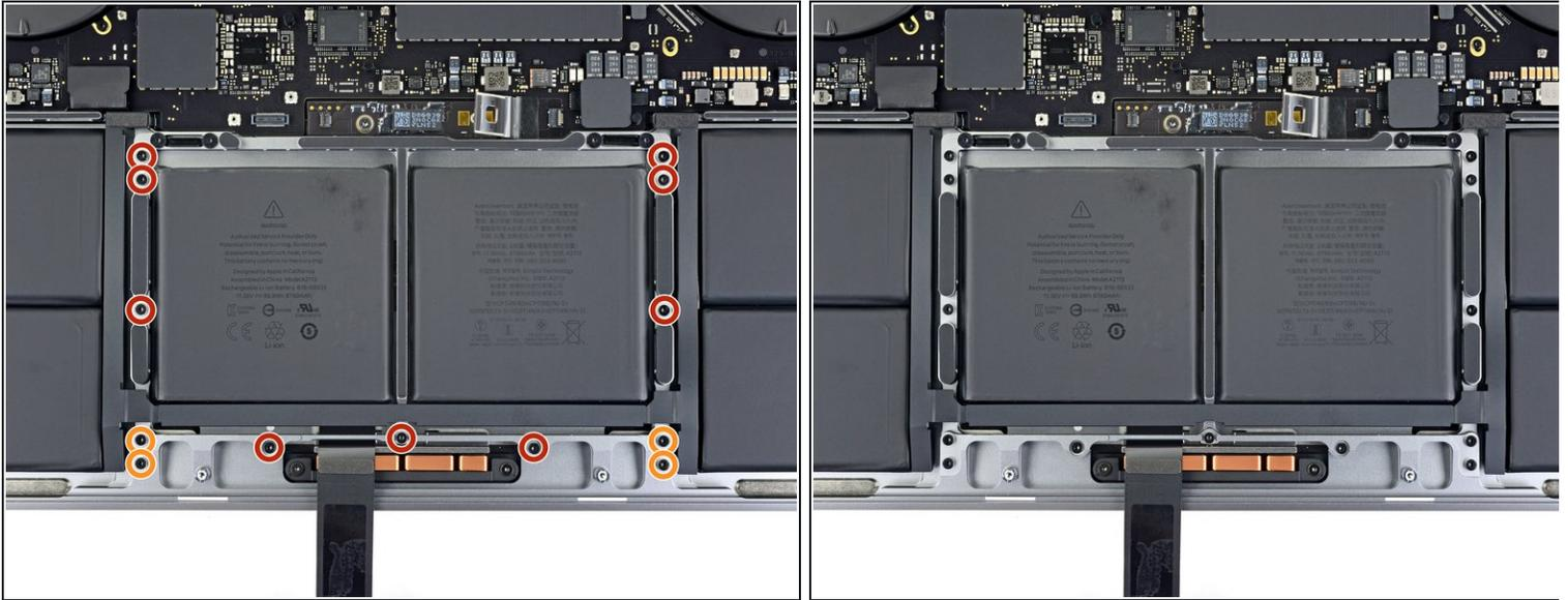
● Use a T5 Torx driver to remove the 13 screws securing the trackpad assembly:
