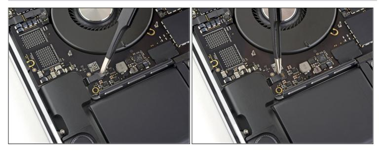
• Peel back any tape covering the left speaker cable connector.
