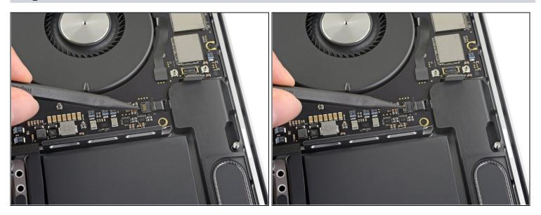
Open the locking flap on the right speaker cable's ZIF connector by prying it straight up from the logic board.
