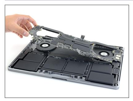
• Lifting from the left side, remove the logic board.
