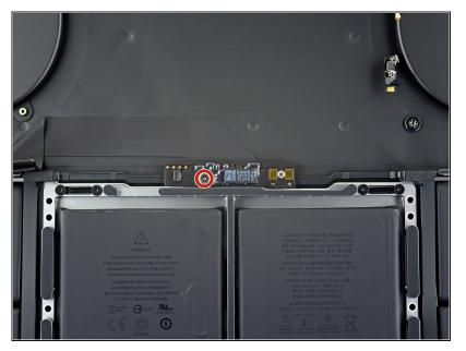
Use a T5 Torx driver to remove the 5.1 mm screw securing the battery board.
