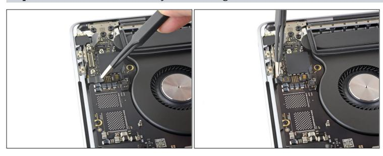
• Peel back any tape covering the other keyboard backlight connector.
