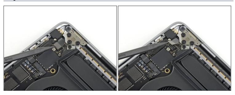
• Disconnect the headphone jack flex connector by prying it straight up from the logic board.
