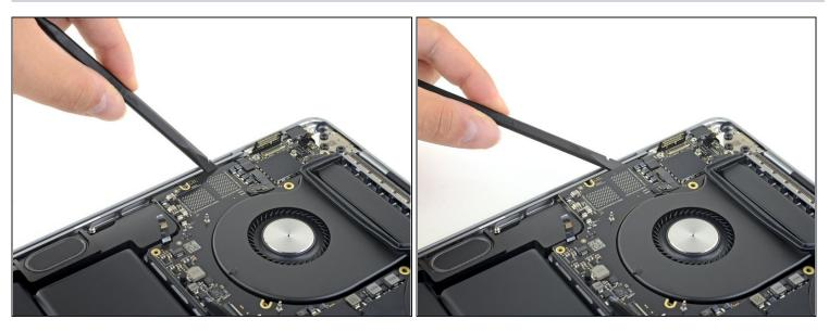
(i) The logic board assembly is a tight fit, but you can make it easier to remove by inserting a spudger under the left edge and levering it up **slightly**.
