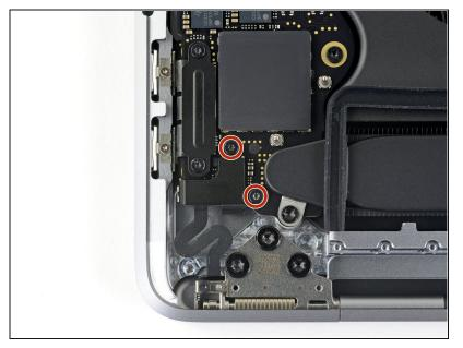
Using a T3 Torx driver, remove the two 1.5 mm screws securing the cover bracket for the Touch Bar digitizer and lid angle sensor connectors.
