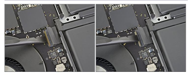
• Use a spudger to gently pry straight up on the long locking flap on the <u>ZIF connector</u> for the keyboard cable.
