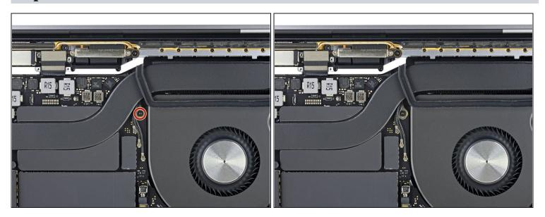
• Use a T5 Torx driver to remove the single 2.9 mm screw securing the antenna cable bundle.
