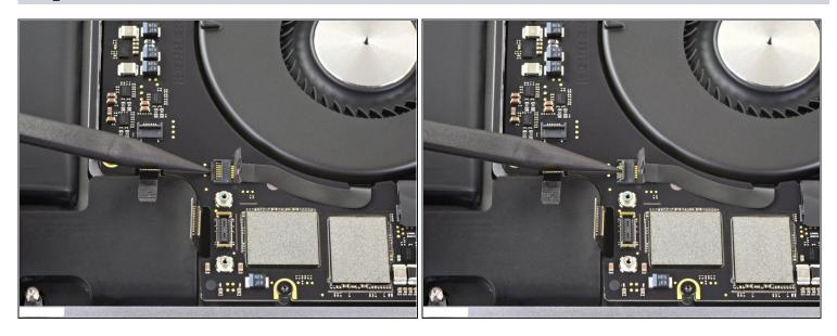
• Open the locking flap on the keyboard backlight's ZIF connector by prying it straight up from the logic board.
