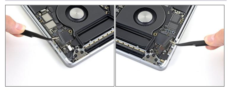
• Remove the cover brackets from both Thunderbolt cable sockets.
