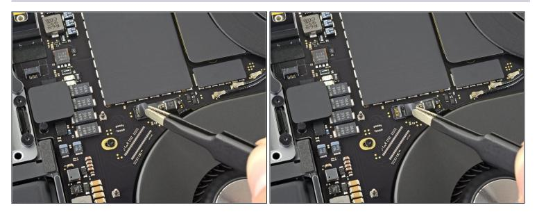
Peel back any tape covering the right fan connector.
