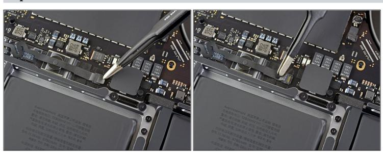
• Peel back any tape covering the battery board data cable connector.
