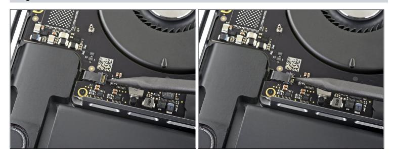
• Open the locking flap on the left speaker cable's ZIF connector by prying it straight up from the logic board.
