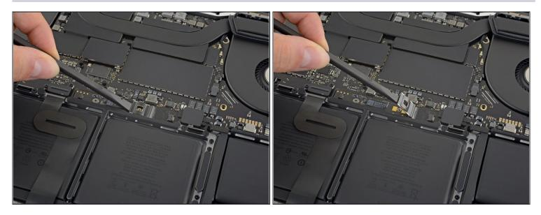
• Use a spudger to lift the battery power connector, disconnecting the battery.
