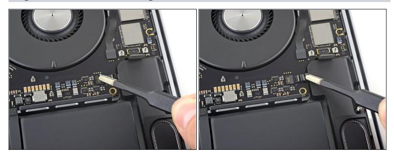
• Peel back any tape covering the right speaker cable connector.
