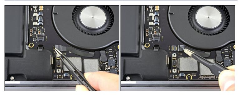
• Peel back any tape covering the first keyboard backlight cable connector.
