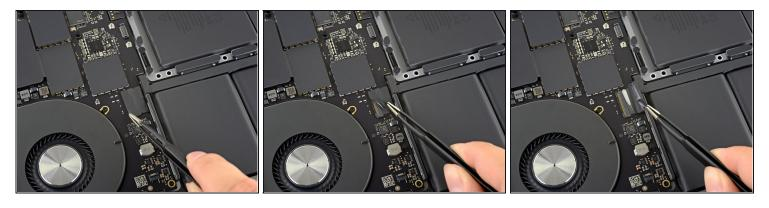
Peel back the tape covering the keyboard cable connector.
