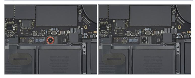
• Use a T5 Torx driver to remove the 6.7 mm pancake screw securing the battery power connector.
