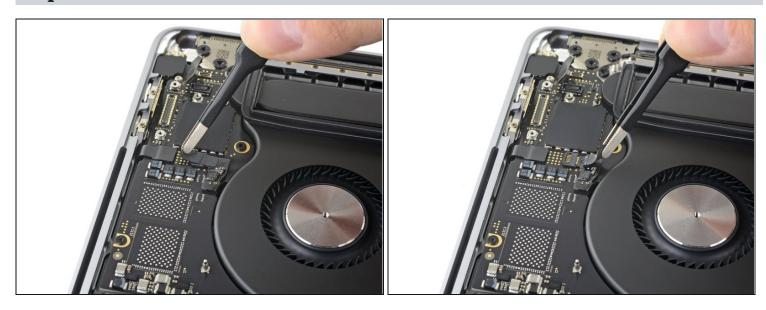
• Peel back any tape covering the left fan connector.
