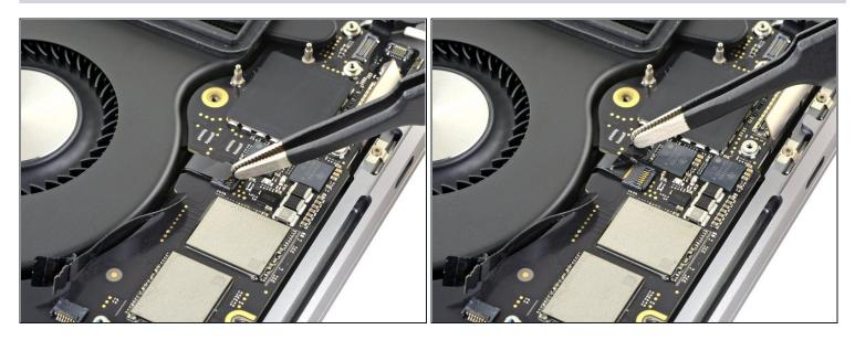
• Peel back any tape covering the microphone array connector.
