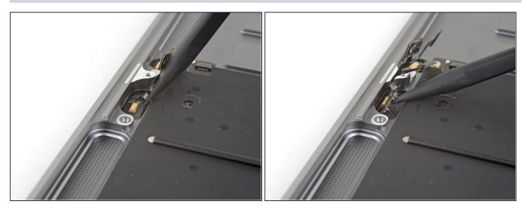
• Use the point of a spudger to carefully pry one of the microphones out of its recess in the upper case.
