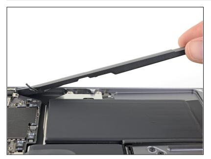
• Lift the left speaker straight up from the bottom and remove it.
