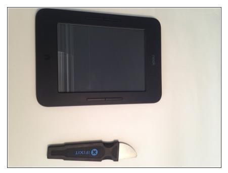
This is the Nook Glowlight 3. It features an E-ink display with a resolution of 300 ppi. This device is touchscreen. It comes with 8GB of on device storage. It is wifi compatible
