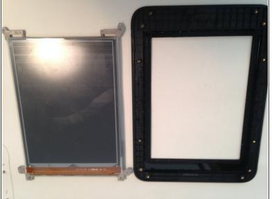
Push firmly on the display. Going all around the edges until the display becomes loose. (the screen was already cracked)
