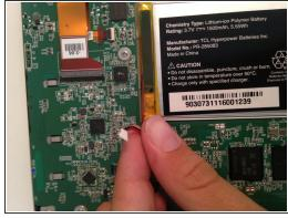
Disconnect the battery with a flick of the spudger.
