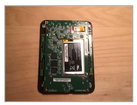
Remove the screws marked in red that secure the system board to the outer plastic.
