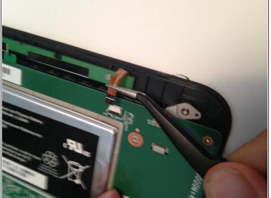
On both sides, there are two straight and skinny button panels. These control the side up/down buttons. Please disconnect both of these ribbon cables.
