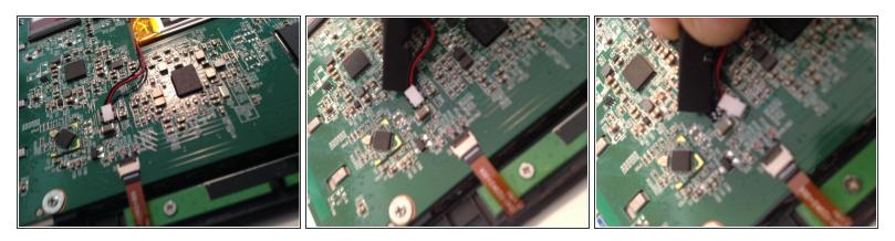
• Disconnect the battery with a flick of the spudger.
