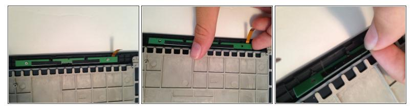
On both sides, there are two straight and skinny button panels. These control the side up/down buttons. Please disconnect both of these ribbon cables.
