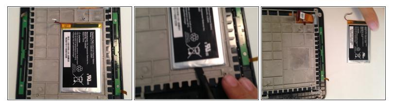
• Now remove the battery by sliding a spudger underneath the battery and breaking the adhesive.
