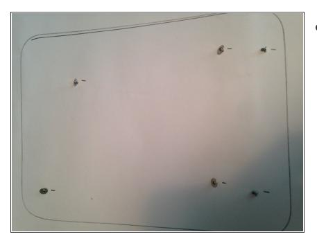
• Tip: Before removing screws draw an outline of the device and place the screws where they are located on the device.
