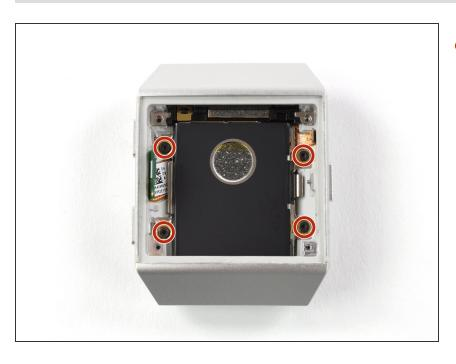
Remove the four Torx T2 screws (1.8 mm length).
