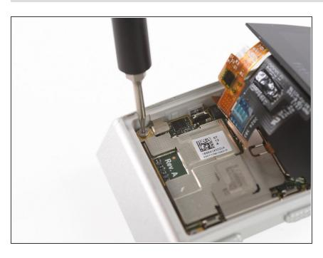
Remove the Torx T2 screw (3.65 mm length) on the bottom left corner.
