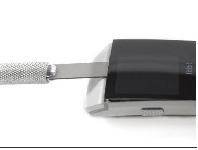
Use a technician's razor with a flat blade to pry up the top edge of the display and create a small gap.
