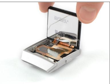
Carefully fold the display assembly in the direction of the bottom edge.
