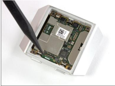
Use a spudger to pry up and disconnect the heart rate sensor from the motherboard.
