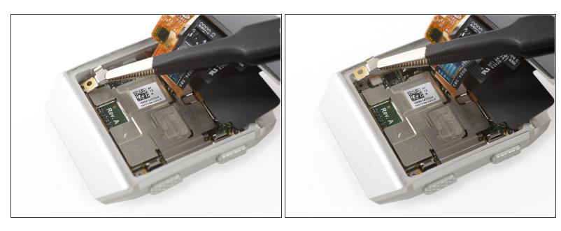
Use a pair of tweezers to remove the metal shield covering the battery flex cable.
