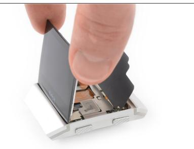
Fold the display assembly back to its original position.
