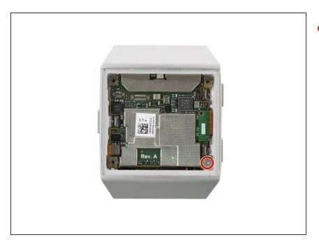
Remove the Torx T2 screw (3.65 mm length).
