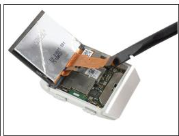
Use a spudger to pry up and disconnect the two display cables from the motherboard.
