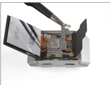
Use a pair of tweezers to remove the metal cover.
