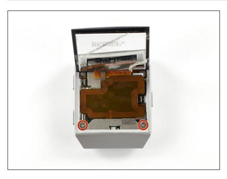
Remove the two Torx T2 screws
