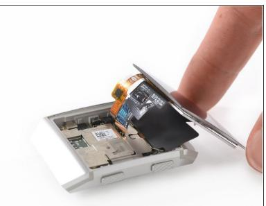
Carefully fold the display assembly onto the upper side of the watch.
