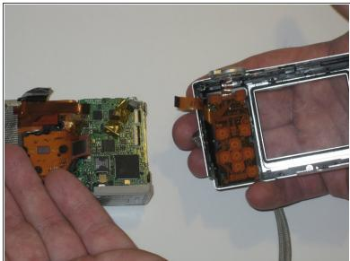
Pull on the shutter button display data cable on the end connected to the motherboard until it slides out.
