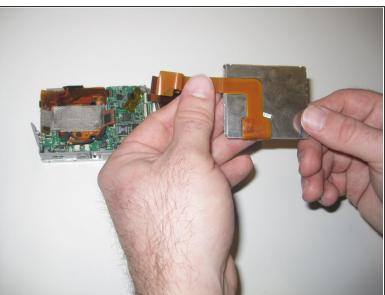
Gently remove the LCD display data cable by gripping the end that is connected to the motherboard and pulling out.
