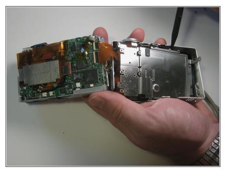
• Slide casing out using the spudger.
