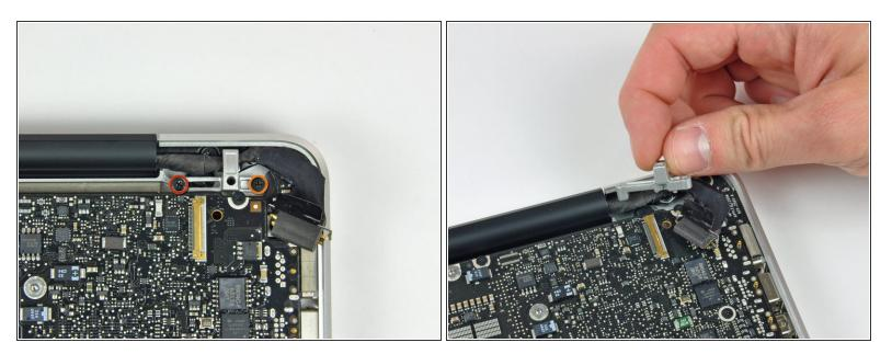
• Remove the following two screws securing the display data cable bracket to the upper case:
