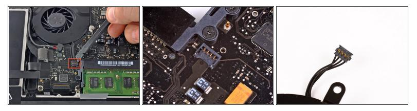
• Use a spudger to pry the fan connector out of its seat, and straight up off the logic board.
