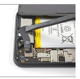
• Using the flat end of a spudger, gently fold the battery cable over so it doesn't accidentally make contact during the rest of your repairs.
