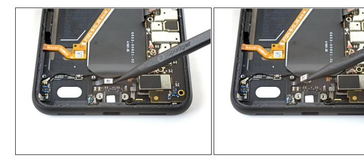
• Disconnect the antenna press connector from the charging assembly.
