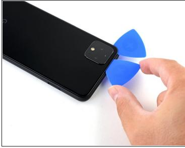
Slide the third opening pick around the top right corner and across the top side of the phone, slicing the final strip of adhesive.
