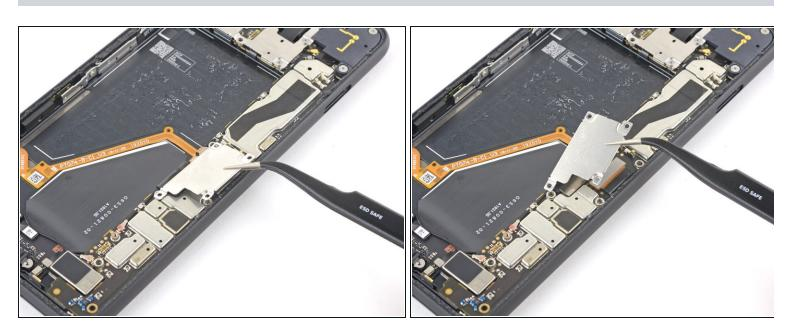
• Use a pair of tweezer to remove the display connector cover.
