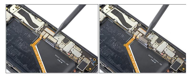
• Using the pointed end of a spudger, disconnect the charging cable connector by prying it straight up from the motherboard.
