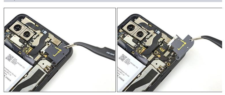
• Use a pair of tweezers to remove the front-facing camera connector cover.
