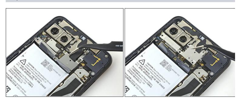
Use a pair of tweezers to remove the rear-facing camera connector cover.
