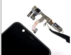
• Use a pair of tweezers to remove the front camera and sensor assembly.
