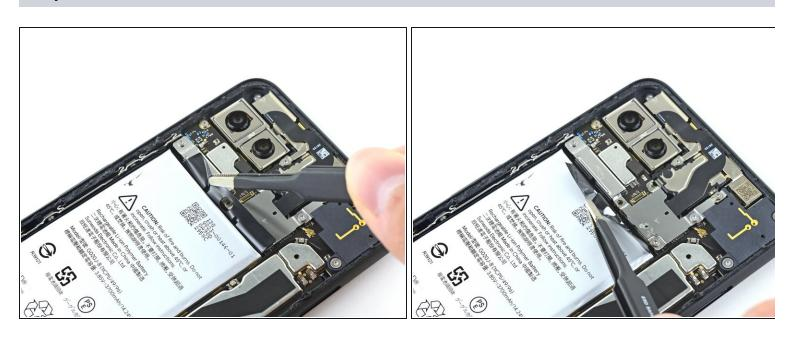
Gently pry back the battery adhesive pull tab to allow easier access to the screws underneath it.
