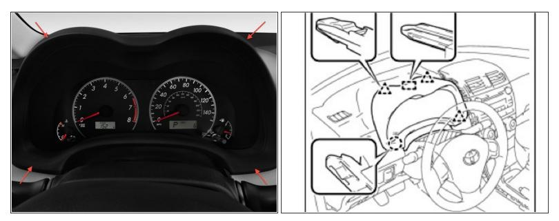
Start by removing the hood over the instrument cluster. Pull the hood straight out towards the steering wheel.
