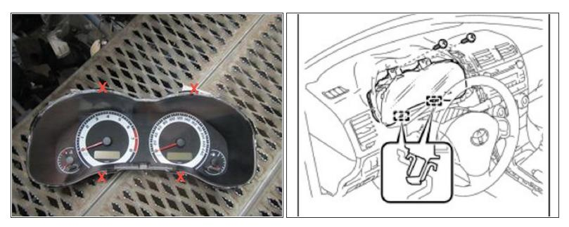
• After removing the hood, undo the four screws securing the instrument cluster and pull forward.
