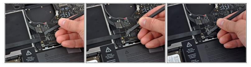
Use the flat end of a spudger to pry the optical drive, hard drive, and trackpad cable connectors up off the logic board.
