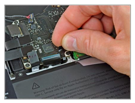
Peel the small strip of black tape off the keyboard backlight ribbon cable socket.
