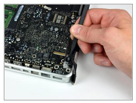
• Use the tip of a spudger to pry the microphone off the adhesive attaching it to the upper case.
