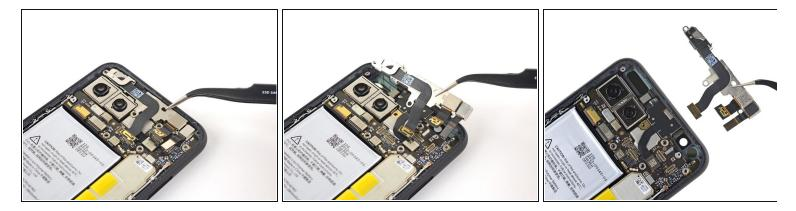
• Use a pair of tweezers to remove the front camera and sensor assembly.
