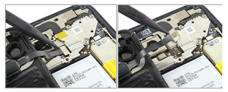
• Using the pointed end of a spudger, pry up and disconnect the back panel connector.
