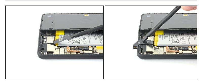
• Using the flat end of a spudger, gently fold the battery cable over so it doesn't accidentally make contact during the rest of your repairs.
