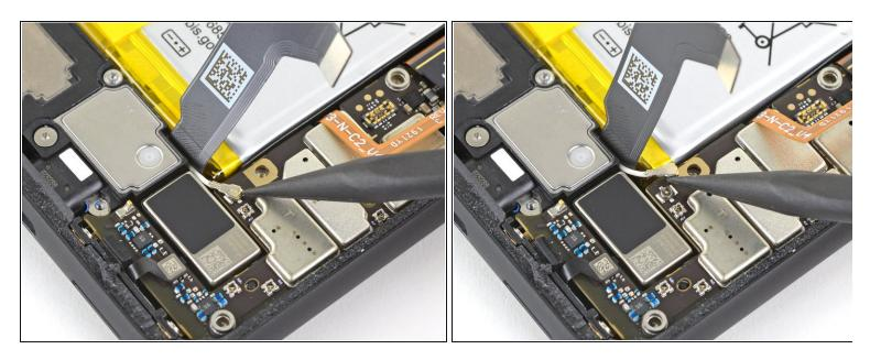
• Use a pair of tweezers to grip the metal clip and pull the connector straight up off of the motherboard
