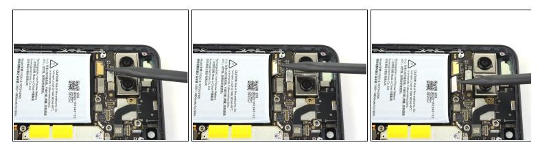
• Use the pointed end of a spudger to disconnect the two rear-facing camera connectors from the motherboard.
