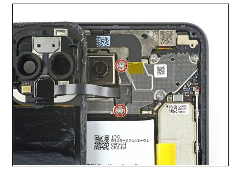
• Use a T3 Torx driver to remove the two 4 mm screws securing the back panel connector cover.
