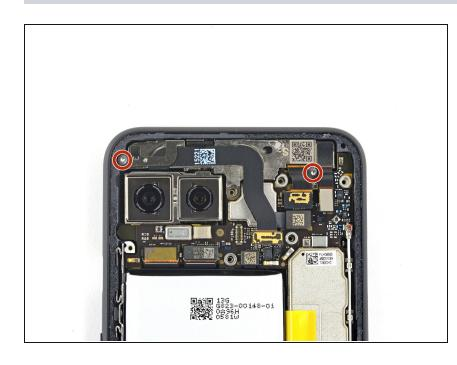
• Use a T3 Torx driver to remove the two 2.4 mm screws securing the front camera and sensor assembly.
