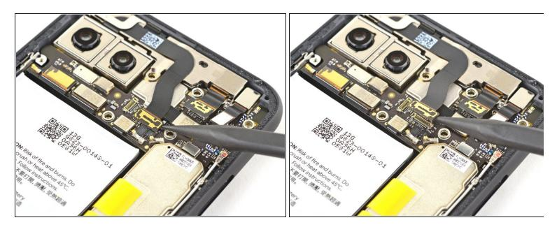
• Disconnect the laser module connector.
