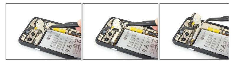
• Using a pair of tweezers, tilt the camera cover up and slide it out of the retaining slot on the upper right corner of the phone to remove.
