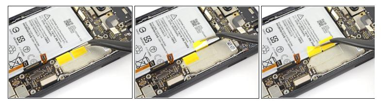
• Gently pry back—but don't remove—the two battery adhesive pull tabs lightly adhered to the motherboard.
